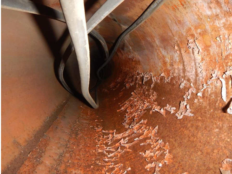
Figure 17. Failed coating on interior surface of pole.
